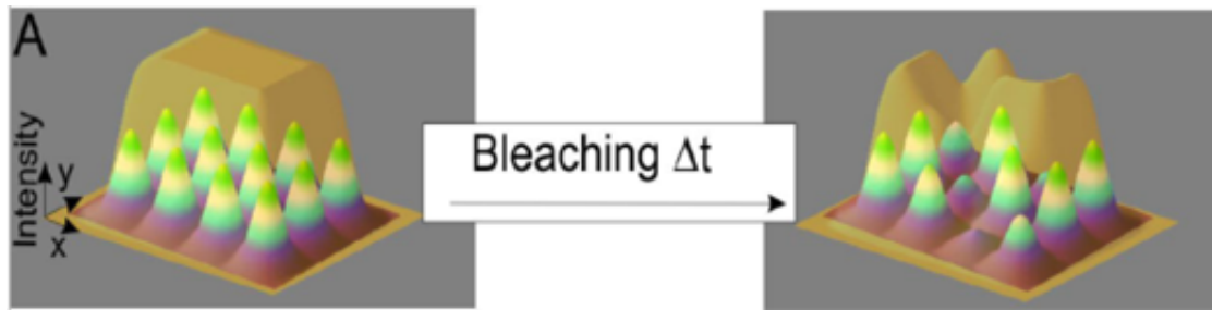
Figure 3.2: Illustration of multiple fluorophores located at the same diffracted limited spot of equal intensity. During imaging, the fluorophores of these complexes bleach and due to statistical uneven bleaching peaks and troughs appear. Reproduced from Figure 1 in [73]
