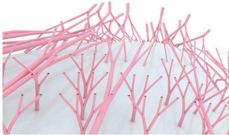
Figure 4.11. Ventilation system predicted using the computer simulation process; Organisation of the Branching Skin with Branching Conduits. 46
