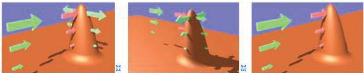
Figure 4.4. The simulation pictures of wind direction and air suction on the membrane of termite mound. 39
