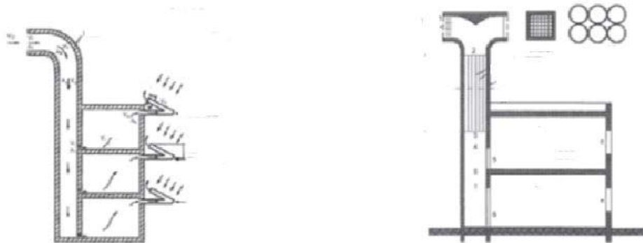
Figure 3.28. (Left) Wind-catcher with solar collector Fig. (Right) Wind-catcher with cooling columns. (Source: Azami A., 2005)
