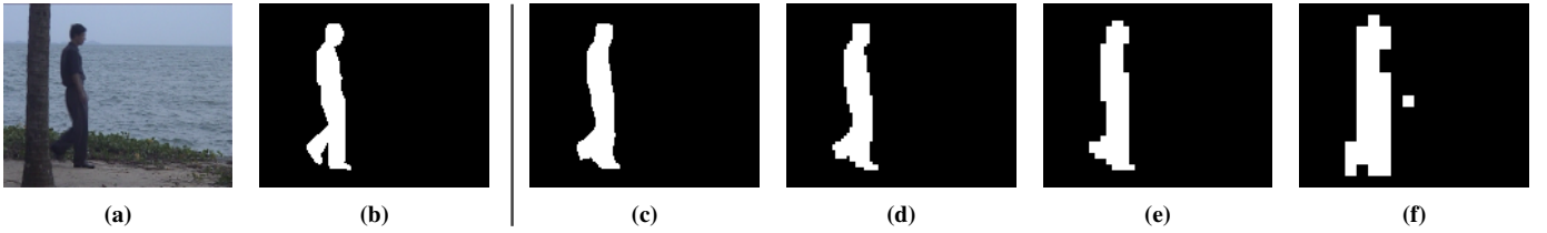
Fig. 2. (a) An example frame from the I2R dataset, (b) its corresponding ground-truth foreground mask. Using the proposed method with a block size of 8 \times 8 , the foreground masks obtained for various degrees of block advancement: (c) 1 pixel, (d) 2 pixels, (e) 4 pixels, and (f) 8 pixels (ie. no overlap).
