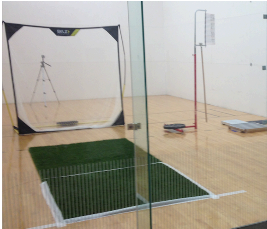
Figure 5. Set-up of kicking velocity test. The ball was placed 3.5 meters in front of the goal (white line) and the speed gun was placed 2.5 meters behind the goal.
