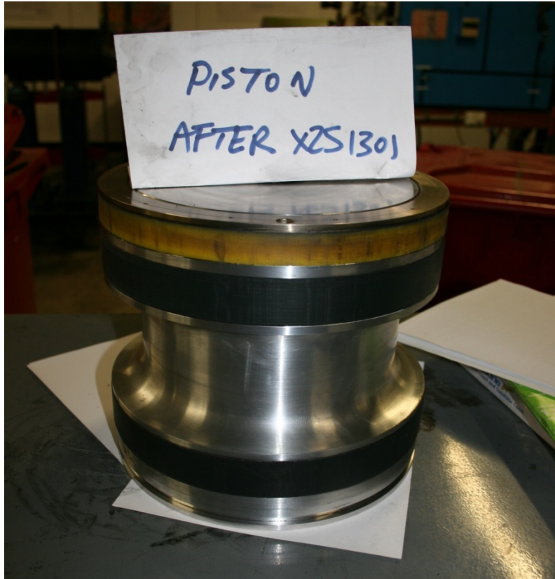
Figure 18: Piston undamaged after 9 shots.
