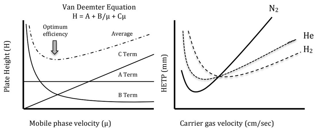
Figure 1-4. The three terms in a Van Deemter plot (left) and the various gases as how they appear in the Van Deemter plot (right).
