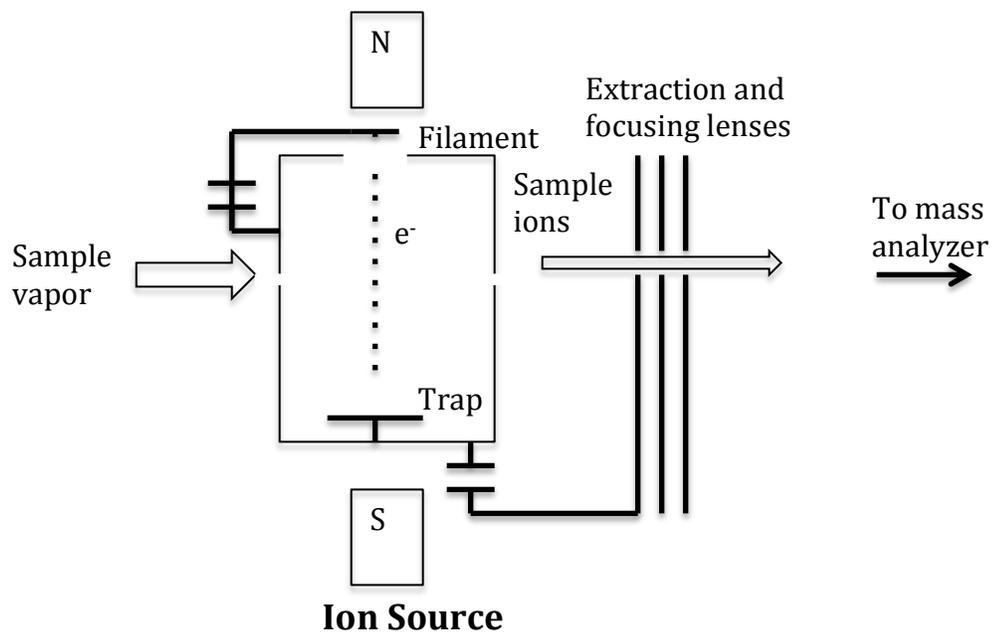
Figure 1-6. Schematic of an electron ionization (EI) source.
