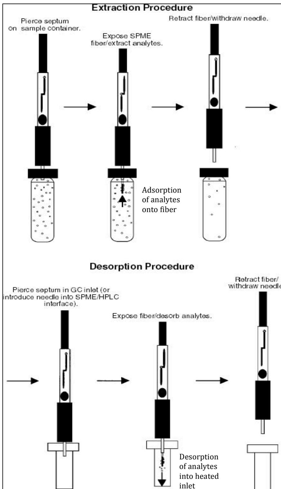
Figure 4-1. Schematic of the direct immersion SPME extraction (top) and desorption (bottom) processes. Adapted from S. Chopra [83].
