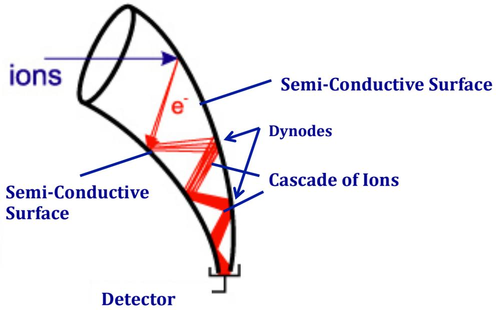
Figure 1-8. Schematic of a continuous dynode electron multiplier. Adapted from J. Benedikt, A. Hecimovic, D. Ellerweg, and A. von Keudell. *J Phys D-Appl Phys.* 45(50) (2012) [62].
