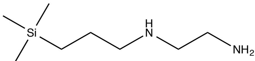
Figure 1-1. Structure of endcapped primary secondary amine (PSA) solid phase extraction (SPE) bulk packing.
