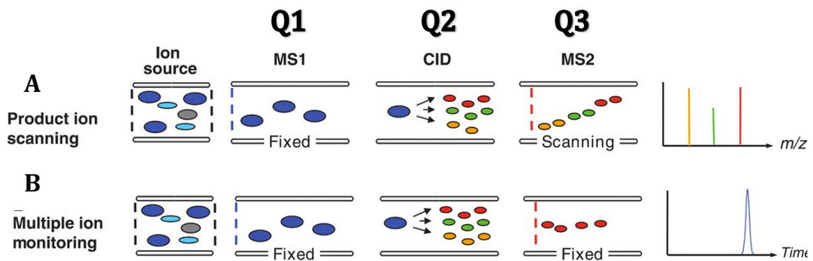
Figure 3-2. Schematic of two triple quadrupole mass spectrometer modes: product ion scan (A) and MRM scan (B). Adapted from [72].
