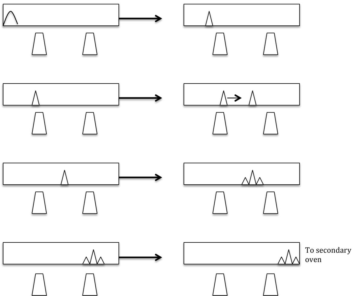
Figure 5-2. Schematic depicting the cryotrap peak modulation process. A) The first cold jet focuses a single component. B) The first hot jet moves the peak to the second cold jet. C) The second cold jet splits the peak of the component. D) The second hot jet moves the peak to the secondary oven.
