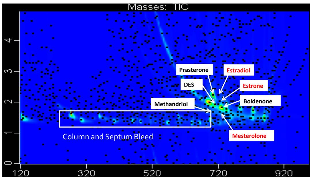
Figure 5-3. Total ion chromatogram of hormones resolved on GCXGC-TOFMS with SPME sample introduction showing the separation of column and septum bleed from the analytes of interest (0.03ppm). Reprinted with permission from Chopra S. Dissertation and Theses 2014 [83].
