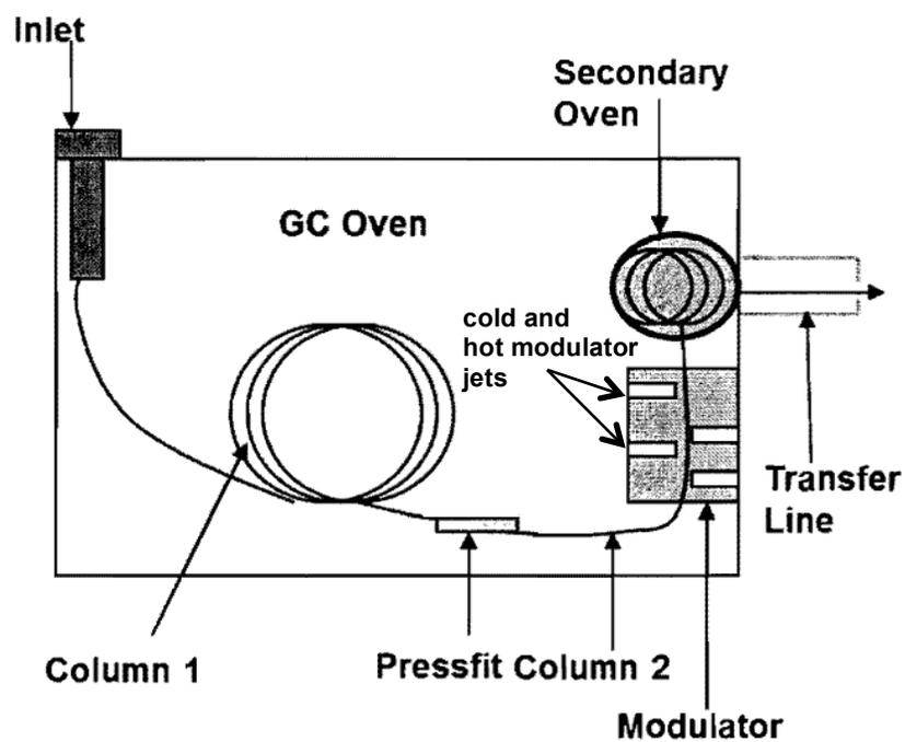
Figure 5-1. Schematic of the GC portion of the instrument used in this research. It can be seen that the second column is housed in a separate oven for heating and a modulator is between the two columns. Adapted from B.B. Barnes 2012 Dissertations Paper 1804 [16].
