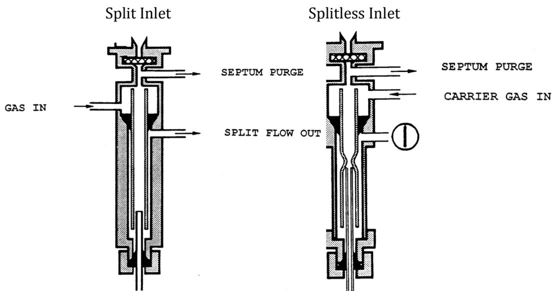
Figure 1-5. Split (left) and splitless (right) injection. Adapted from Y. Kazakevich GC Injectors Lecture Slides [60].
