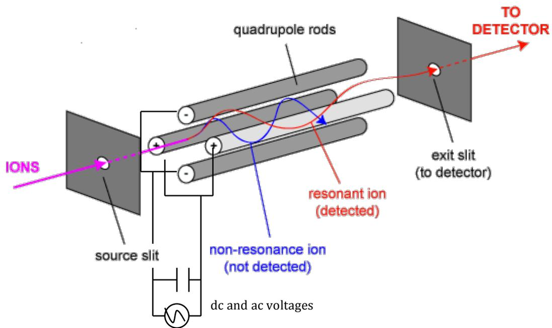
Figure 1-7. Schematic of a quadrupole mass analyzer. Adapted from P. Gates Gas Chromatography Mass Spectrometry (GC/MS): Figure 2 [61].
