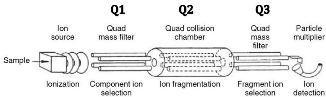
Figure 3-1. Schematic of a triple quadrupole mass spectrometer. Adapted from [71].
