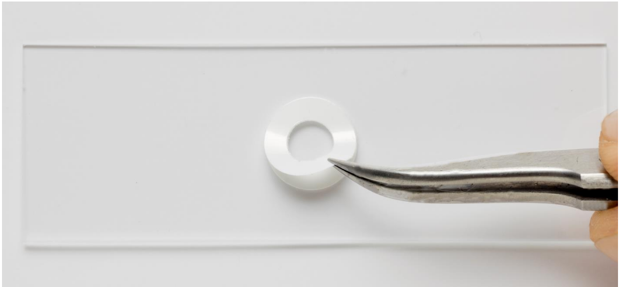
Fig. 4. Preparation of slide using reinforcement rings.
