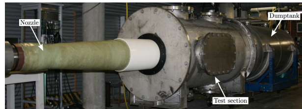
Figure 6: X3 nozzle, test section and dumptank [5]
