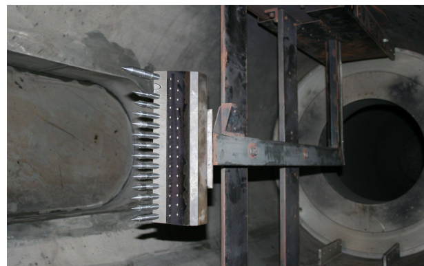
Figure 7: Internal view of X3 test section with pitot rack installed [5]
