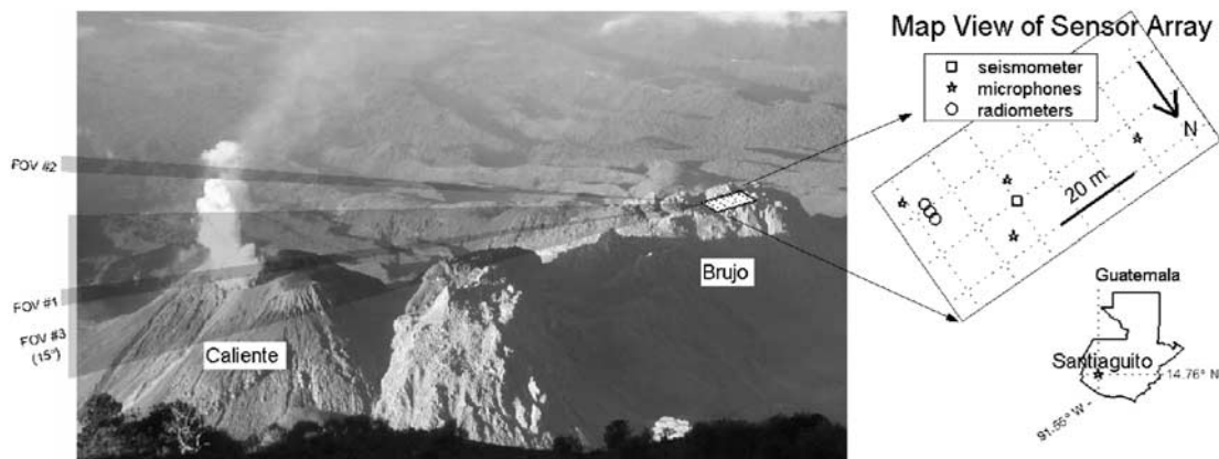
Figure 1. Santiaguito dome viewed from Santa Maria. Active Caliente vent is at left (east) ~1600 m from the inactive Brujo Dome, where sensors (inset map) were installed. Thermometer FOVs are shown as transparent cones.
