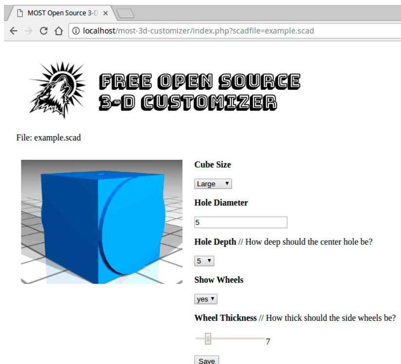
Figure 3. The parameters were adjusted on the Free Open Source 3-D Customizer page to create a new design.
