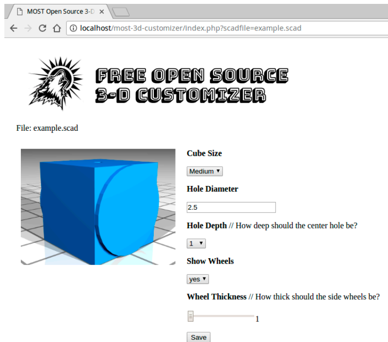
Figure 2. The initial page of Free and Open Source 3-D Customizer loading the example SCAD file from Section 2.3.
