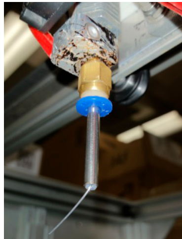
Figure 11. Wire feed guide tube. As shown, a standard M6 4.0 mm press fitting accommodates the standard threading in the hot-zone of a standard hexagon 12 V hot end. 304 stainless tubing press fits similar to a 4.0 mm PTFE tubing. Scrap PTFE tubing is fixtured to the exit zone of the 304 stainless tubing to reduce the friction associated with wire wrapping processes.
