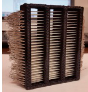
Figure 14. Metal polymer composite generation dimensionally accurate to prescribed models. Cross-flow media is 1100 series aluminum wire, encased in a polymeric matrix of PETG.
