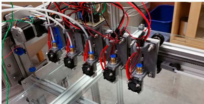
Figure 2. X-axis gantry assembly. 5 × Hexagon Full-Metal 12 V hot ends are shown fixtured to their respective ‘Z-Height Bed Leveling Adjustment’ part files. As shown, dovetail leveling mechanisms are attached to the machined aluminum plate (3.175 mm × 25.4 mm × 295.75 mm) with Hexagon nozzle diameter cylindrical axis spaced 55 mm.
