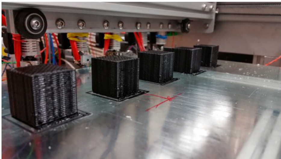
Figure 15. Printed component part quality (visual inspection) prior to removal from substrate to be measured for dimensional precision. As indicated in Table 9, dimensional variation between hot ends is determined to be a critical metric in contrast to print parameter adjustable deviation from nominal dimensional values (i.e., 25.4 mm).
