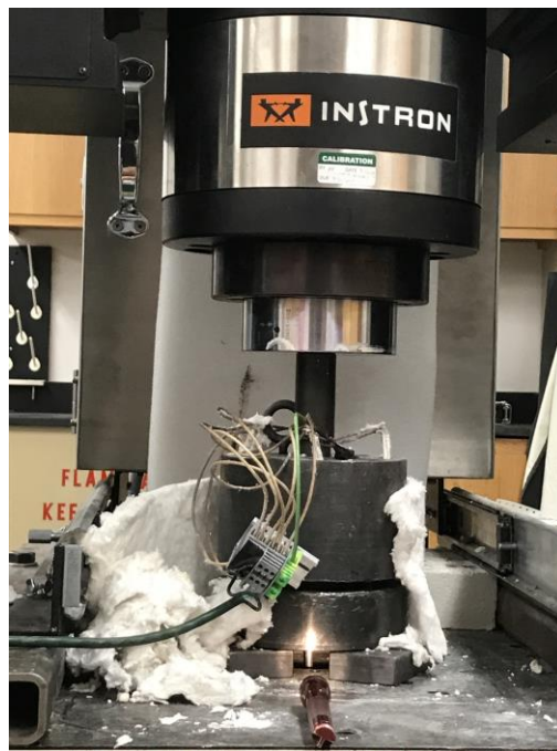
Figure 4.3. System setup used in the hot extrusion process.
