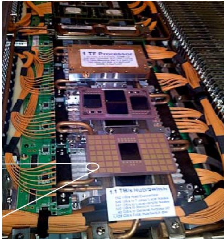
Figure 2: Blue Waters Line Card Demonstrating Fiber Connections [12]
