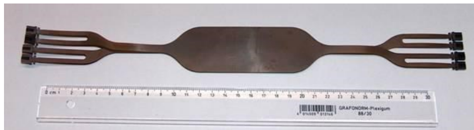
Figure 4: Polymer Waveguide Flex Ribbon Consisting of 8 Polymer Waveguide Layers[19]
