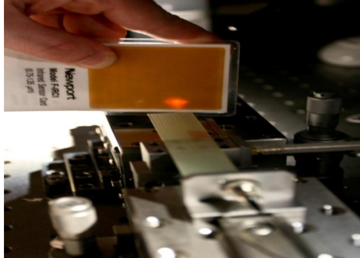
Figure 17: Light Propagation through Waveguide Cladding
