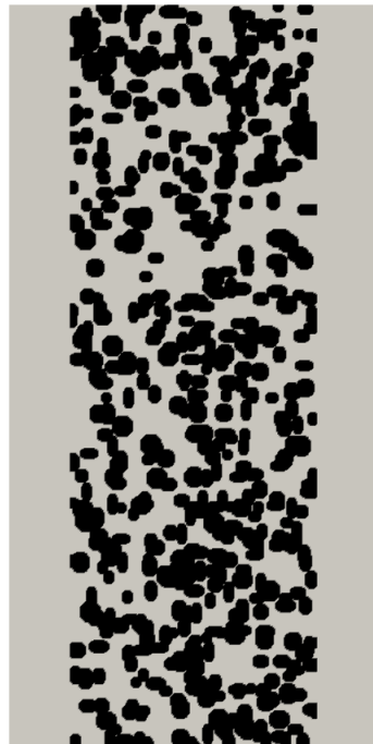
Figure 6.1: Sample generated substrate geometry: 50% porosity.
