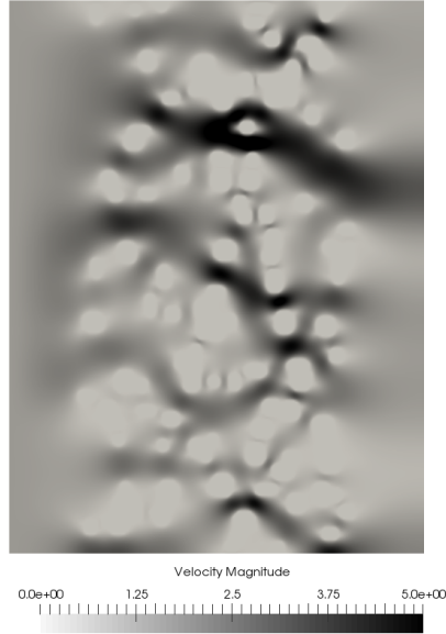
Figure 6.7: Velocity field at 80% porosity ( Re 49).
