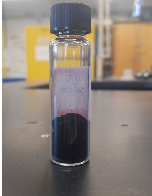
Figure 4-1: Synthesized PEDOT:PSS polymer after 24 hours of polymerization, double filtration and overnight drying.
