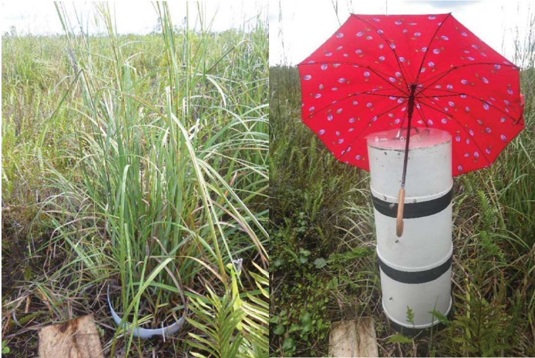
Figure 3. Collar surrounding the culm of sedges in the open peatland (left). PVC extensions used to measure ecosystem gas fluxes (right).
