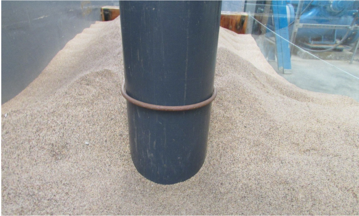
Figure 3. Steel diffuser pipe around the upstream half of the pier (looking downstream)
