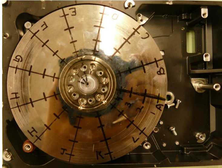
Fig 3.4: The test set-up of the platter used to perform modal analysis. The points from the outer radius to inner radius is named as point 1 to point 4.
