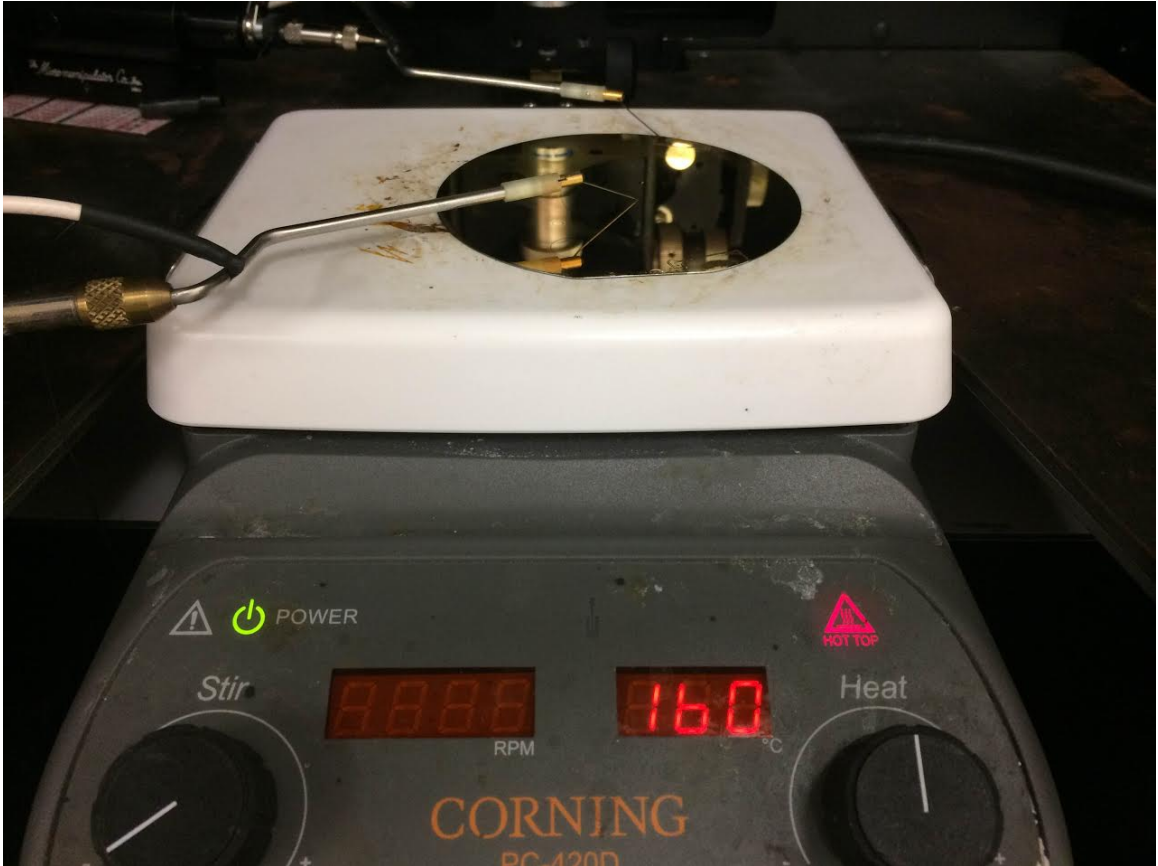
Figure 3.4: Resistivity sample on hot plate at a surface temperature of 135°C during testing
