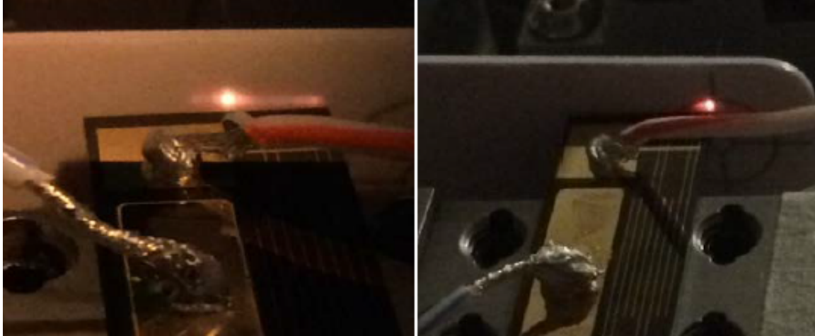
Figure 5.15: Profile of light at output of Mach-Zehnder on infrared detection cards
