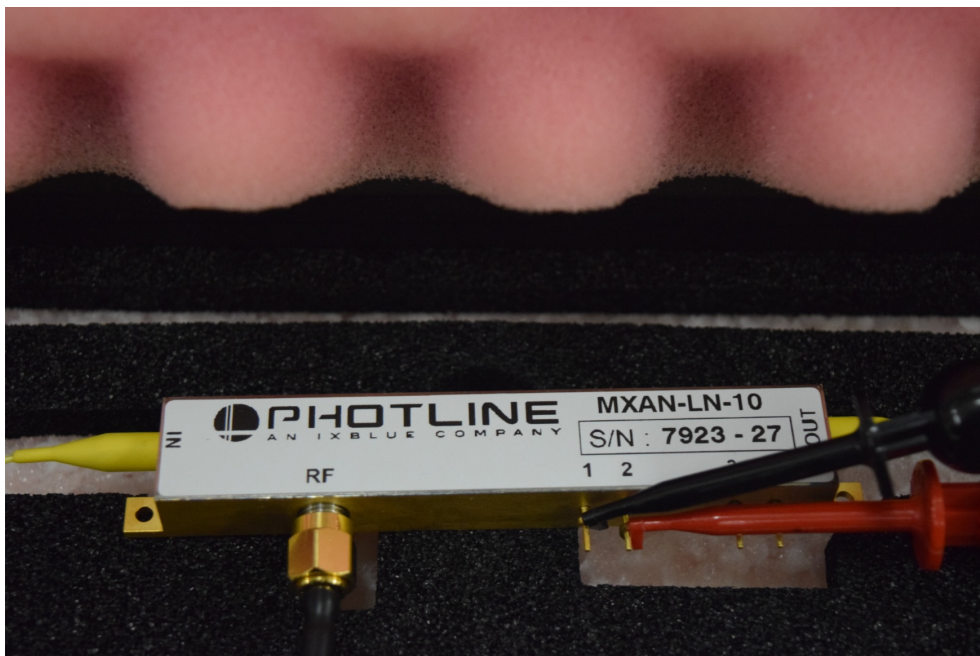
Figure 5.2: Photline MXAN-LN-10 with optical, RF and DC voltage applied
