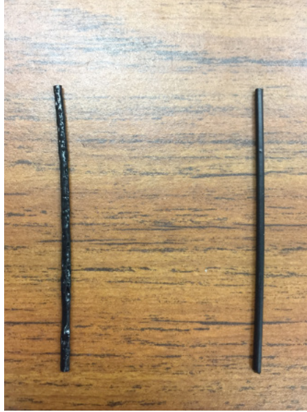
Figure 3.3 Comparison of filament quality from moist pellets and dried pellets
