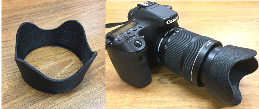
Figure 3.14 The camera hood printed a) with camera and b) with camera by the RepRap from recycled ABS filament
