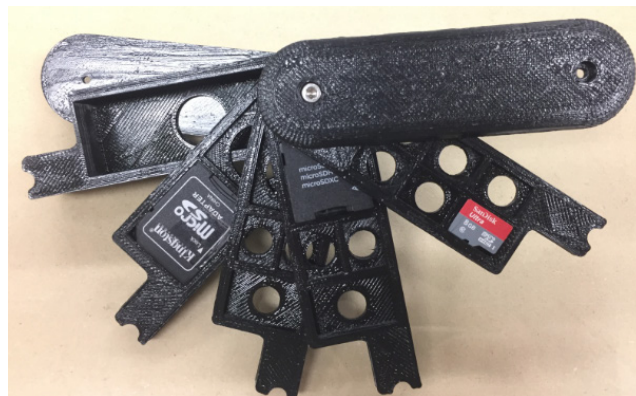
Figure 3.13 The SD card holder printed by the RepRap from recycled ABS filament
