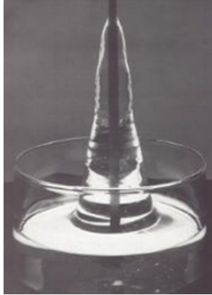
Figure 2.3: The Rod-Climbing effect. Reprinted from An introduction to Rheology, by Barnes, H. A. et al. [115], 1989, Elsevier, p. 61. Copyright 1989, with permission from Elsevier. See documentation in Appendix B.
