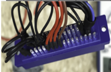
Figure 7. 50 pin Honda Tsushin Kogyo MR-50RFD connector with detailed pin assignments
