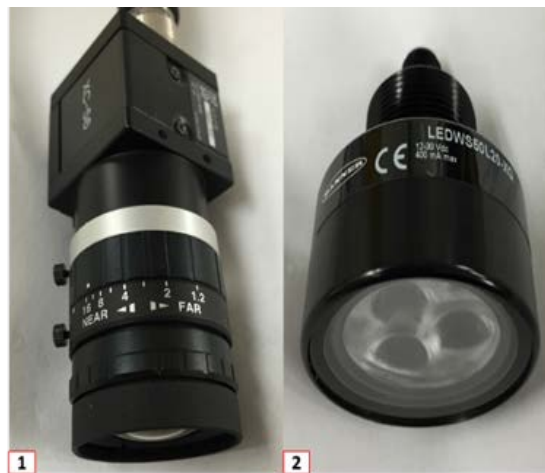
Figure 2. 1) XC-56 Sony Camera 2) LED spot light. These are connected to the robot's controller.
