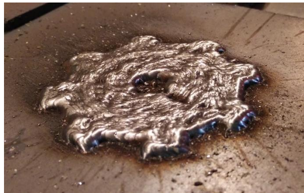
Figure 3.10 The result of printed gear (60 mm diameter) with 2 mm layer height.
