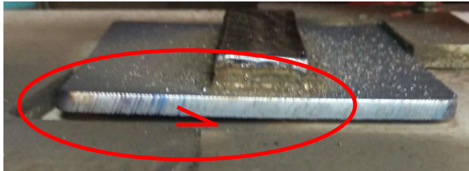
Figure 3.18 Thermal induced substrate deformation which is indicated by the angle symbol (101.6 mm \times 31.75 mm).
