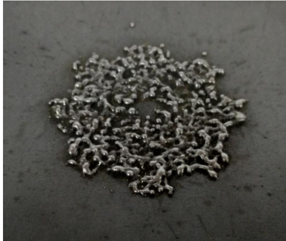
Figure 3.9 The result of printed gear (60 mm diameter) with 1 mm layer height.
