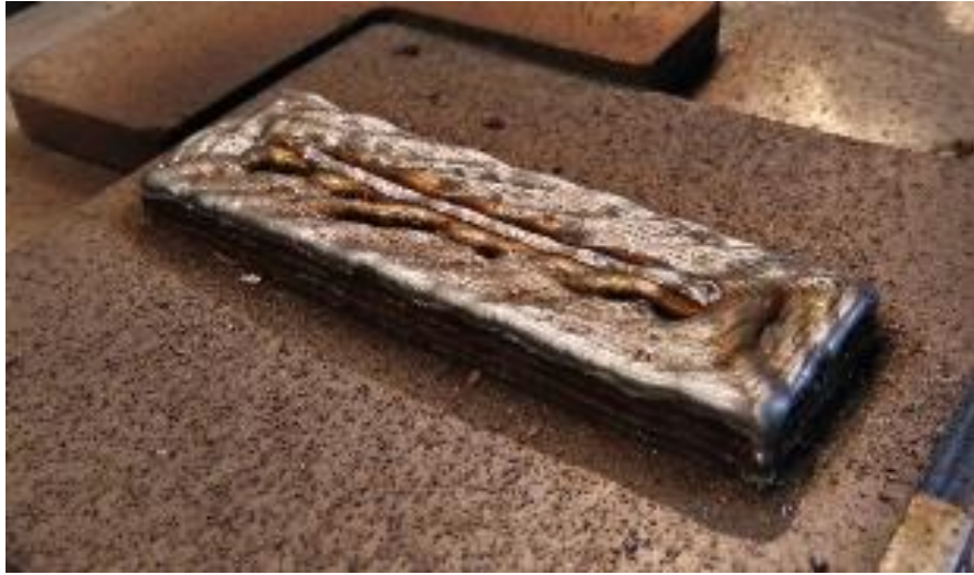
Figure 3.11 Poor surface quality after third layer of printing speed 10 mm/s on block (101.6 mm \times 31.75 mm).
