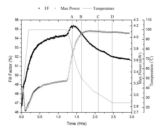
**Figure 3:** High-temperature annealing pulses (spike annealing) results for 25 °C degradation showing the fill factor, maximum power and temperature (A: 80 °C, B: 50 °C, C: fan turned on, D: 25 °C) as a function of time.
