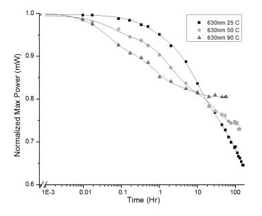
**Figure 2:** A normalized temperature series of 25, 50 and 90 °C degradation under 1 sun for a PV cell with an i-layer thickness of 630 nm.
