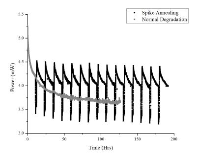
**Figure 7:** Comparison of the same 630 nm i-layer thick a-Si:H PV cell degraded at 50 °C under 1 sun (Normal Degradation) to results obtained for degradation at 50 °C under 1 sun coupled with spike annealing at 100°C on a 12 hour cycle for 192 hours (Spike Annealing).
