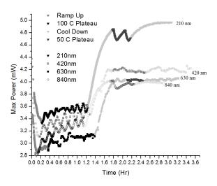
**Figure 6:** High-temperature annealing pulses (spike annealing) thickness series showing the maximum power as a function of time using a-Si:H cells with i-layer thicknesses of 210, 420, 630 and 840nm degraded at 50 °C under 1 sun. The color of the symbols indicates the stage of the temperature cycle.
