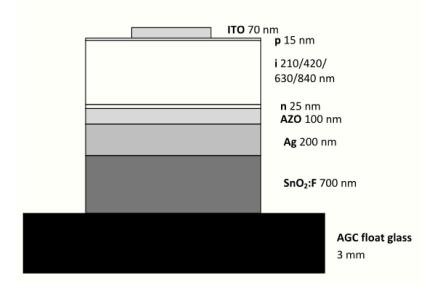
Figure 1: The composition and structure of the a-Si:H solar photovoltaic cells used in this study.
