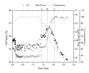
**Figure 5:** High-temperature annealing pulses (spike annealing) results for 90 °C degradation showing the fill factor, maximum power and temperature (A: 90 °C, B: 80 °C, C: 50 °C) as a function of time.
