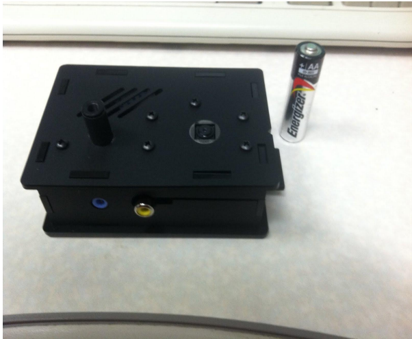
Figure 3. MLX90614ESF-BCI-000-TU-ND sensor, Pi-NoIR, and Raspberry Pi in a Nwazet Pi Camera Box
