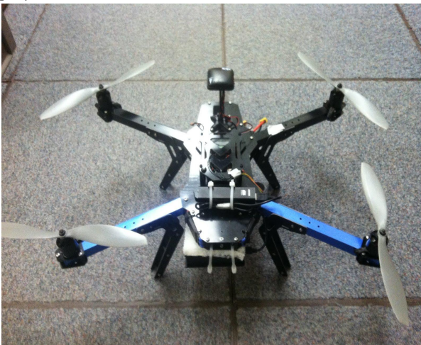
Figure 2. Close-up image of the top of the 3D Robotics Quad platform.
