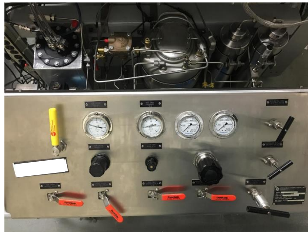
Figure 17: Diesel injection system in CV lab
