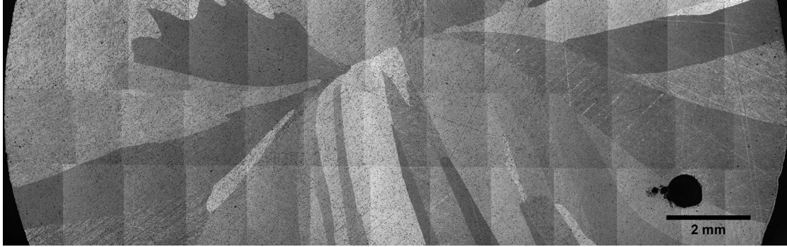
Figure 23: Stitched macrograph of 99.99% Al for grain size measurements
