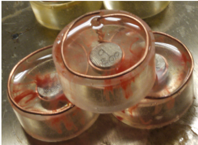
Figure A1: Mounted sample of aged, swaged, and annealed LP09 (Al-0.08 Zr-0.07 Ti) with wire incorporated into mount for anodizing and electropolishing.
