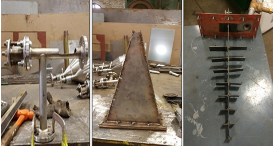
Figure 3-4-(Starting from left to right)-Modified dosing auger body for new feed hopper, modified feed hopper with 75° inclination and new agitator.
