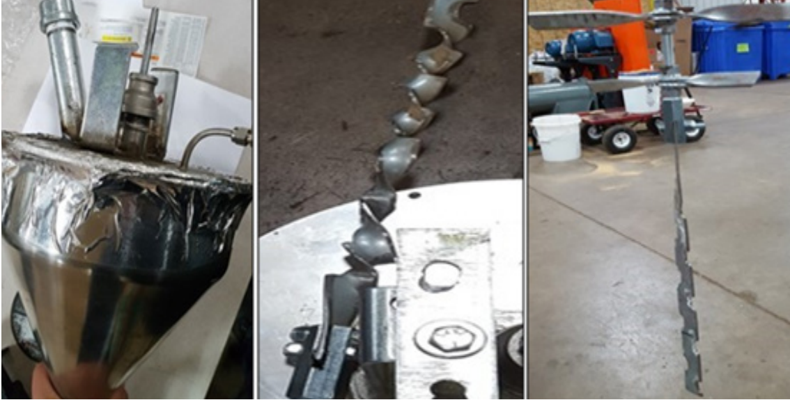
Figure 3-3- (Starting from left to right)-The old hopper with agitator, The old agitator with a bend and The old agitator.
