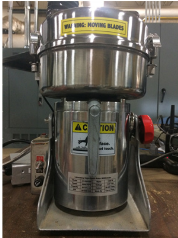
Figure B-1-Laboratory high-speed rotor mill/grinder.
