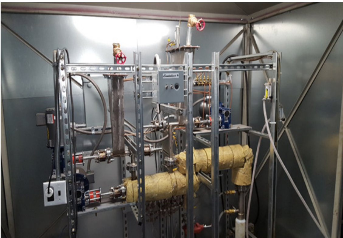
Figure 3-1-Fast pyrolysis unit at MTU.
