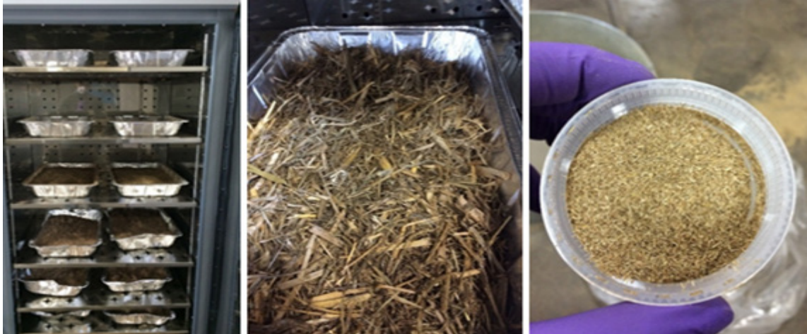
Figure 3-10- (Starting from left to right)-Arundo Donax drying on the oven, raw Arundo Donax and grinded and sieved Arundo Donax.
