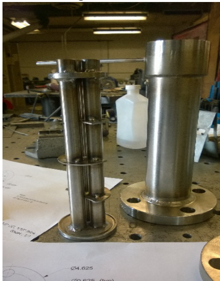
Figure 3-8-Shell tube heat exchanger with baffles on the tube side.
