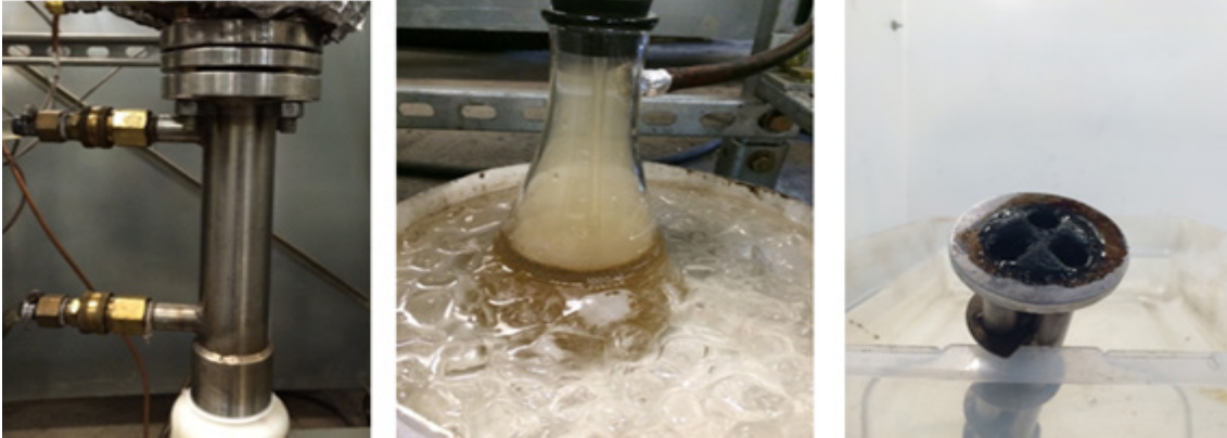
Figure 3-9- (Starting from left to right)-The condenser image, scrubber and tube side of heat exchanger with condensed bio-oil on the top.
