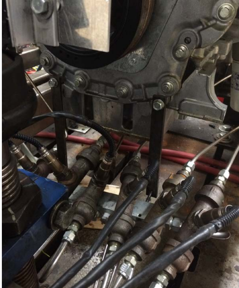
Figure 3- Six individual wide-band sensors mounted on pipes which come from exhaust manifolds of both banks
