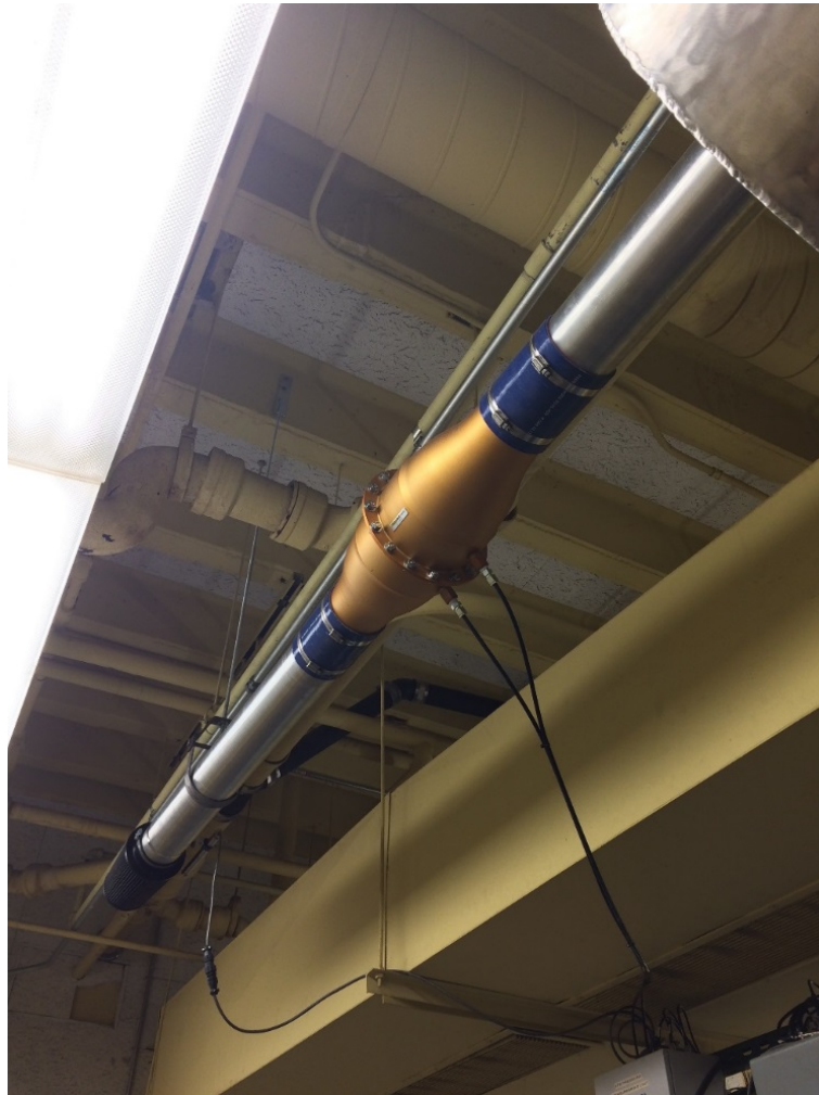
Figure 5- Laminar Flow Element (LFE) setup mounted on intake pathway to the engine
