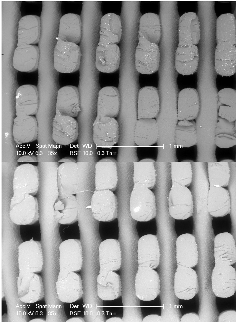
Figure 6.9: The surface of the fracture interface of 1 hour annealed (top) and unannealed (bottom) samples, taken with an Environmental Electron Scanning Microscope (ESEM).
