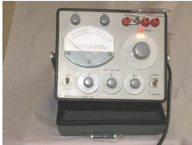
Figure 1. 3 1864 megohmmeter for electrical resistance measurement.
