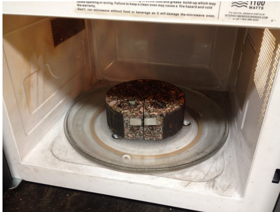
Figure 9. 4 Microwave healing of asphalt mixture sample.
