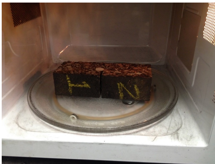
Figure 4. 5 Microwave healing of asphalt mixture beam sample.
