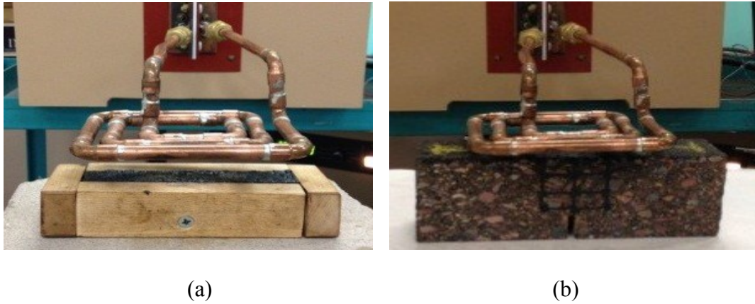
Figure 2. 2 Induction heating system with heating generator and induction coils: (a) asphalt concrete sample healing and; (b) asphalt mastic sample healing.
