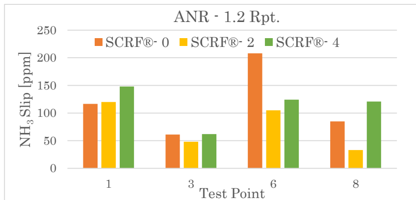
Figure 3.8 NH 3 slip from SCR F ® for NO x reduction test points at ANR - 1.2 Repeat (Rpt.)
