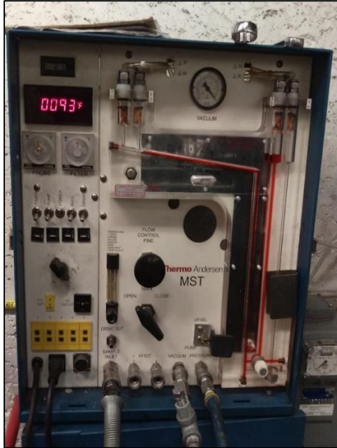
Figure A.1 Manual Sampling Train
