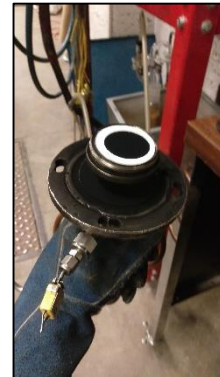
Figure A.3 a) PM sampling probe (left picture) b) Filter paper (right picture)
