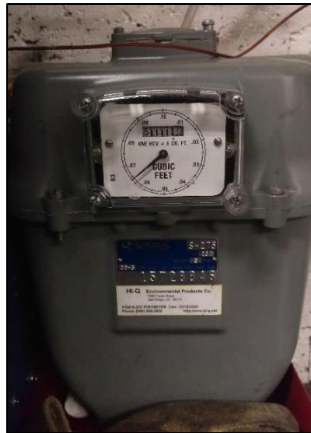
Figure A.2 Dry Gas Meter
