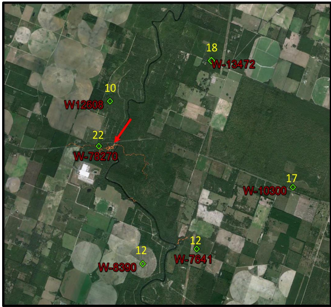
Figure 2: Map showing water wells near Madison Blue Spring State Park. The red numbers are the well identification number and the yellow numbers indicate the bedrock elevation in each well. These wells show that regionally the bedrock is practically flat having a maximum dip of 1.3 degrees between wells 78270 and 12608. Well number 78270 also indicates a water table elevation of 15.5 meters which is useful in determining the proximity of the water table and bedrock at the nearby study location indicated by the red arrow.
