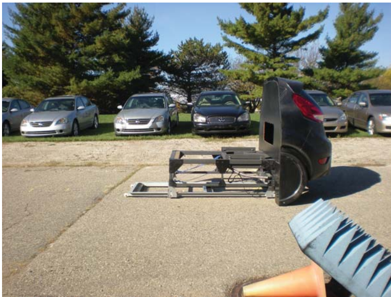
Figure 46: NHTSA SS_V2 Test Surrogate - Side View. In the foreground is an orange pylon supporting radar absorbing tile to reduce high clutter response from a manhole cover with an elevated rim.
