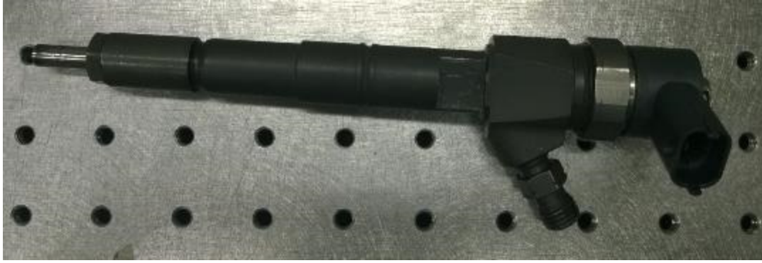
Figure 3-7: Bosch HPCR solenoid type injector with 200 micron nozzle hole diameter
