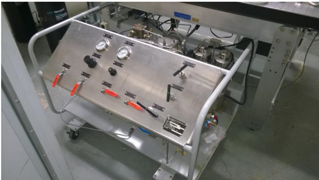
Figure 3-8: Fuel pump system used to pressurized injector
