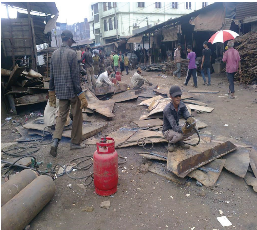
Figure 2.3: Old Dhaka steel plate processing by cutter men, using gas torches powered by cylindered gases (Photo Credit; First Author).
