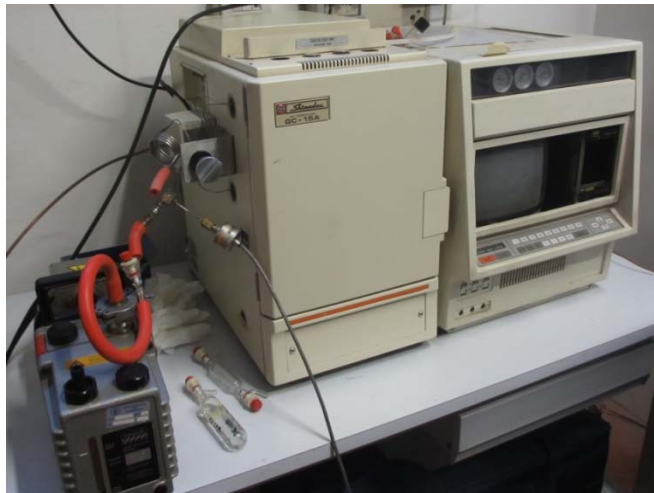
Fig. 6, Gas chromatograph Shimadzu 15A for the analysis of H_2 , Ar, He, Ne, O_2 , N_2 , and CO content
