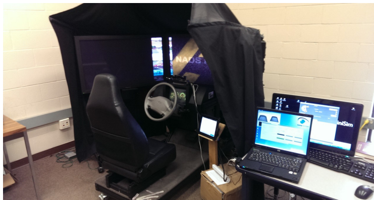
Figure 13. Equipment setup, featuring the NADS simulator, and a laptop for recording the two webcams.
