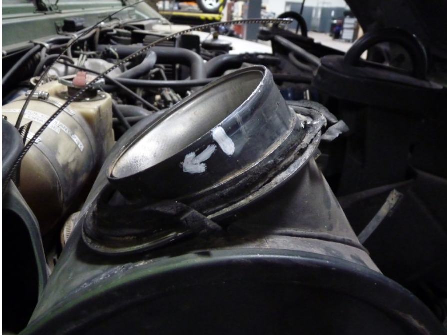
Figure 6.3: Inlet of HMMWV air filter with marks showing where to block off with tape. The tape should go on the side of the line with the arrow. There is another line and arrow on the hidden side of the inlet.
