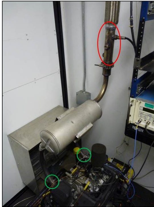
Figure 4.15: Picture of exhaust system in front test cell. Thermocouple bung locations are circled in green. O 2 sensor bung locations are circled in red.
