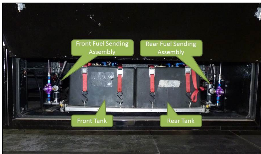
Figure 4.3: Picture of the Mobile Lab fuel system in the trailer belly box.
