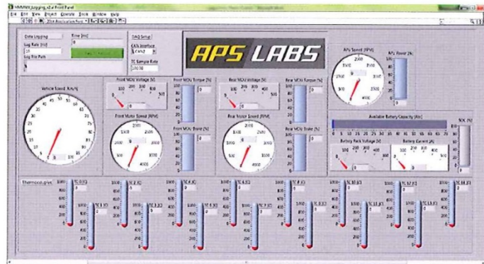
Figure Error! No text of specified style in document..23: Virtual instrument front panel for logging data on the HE-HMMWV.
