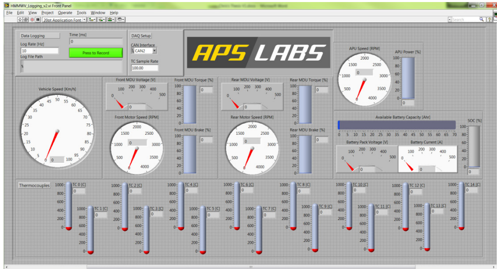
Figure 6.2: Virtual instrument front panel for logging data on the HE-HMMWV. This image contains content under copyright ownership of NI. Use of this material is courtesy of NI according to the agreement found in Appendix B.
