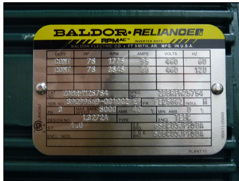
Figure 4.10: Image of nameplate for Baldor Reliance motor
