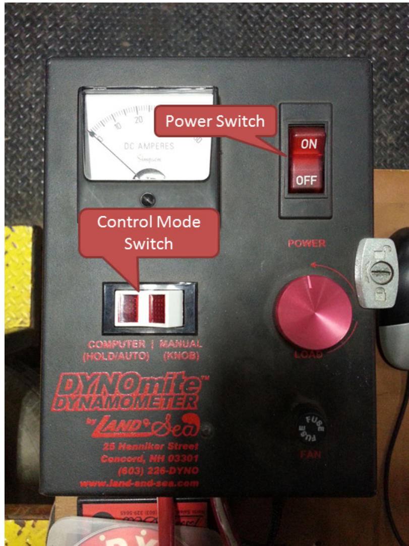
Figure 6.8: Picture of the front of the dyno servo control box. The power and control mode switches are shown.
