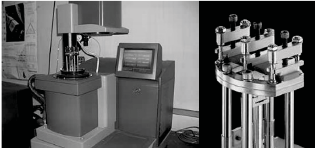
Figure 3-11: left) TA Instruments Q800 DMA right) Dual/single cantilever clamp
