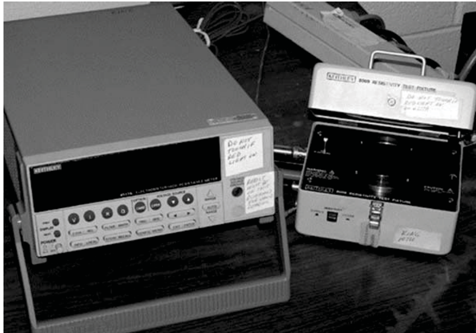
Figure 3-9: (left) Keithley 6517A Electrometer/High Resistance Meter, (right) Keithley 8009 Resistivity Test Fixture
