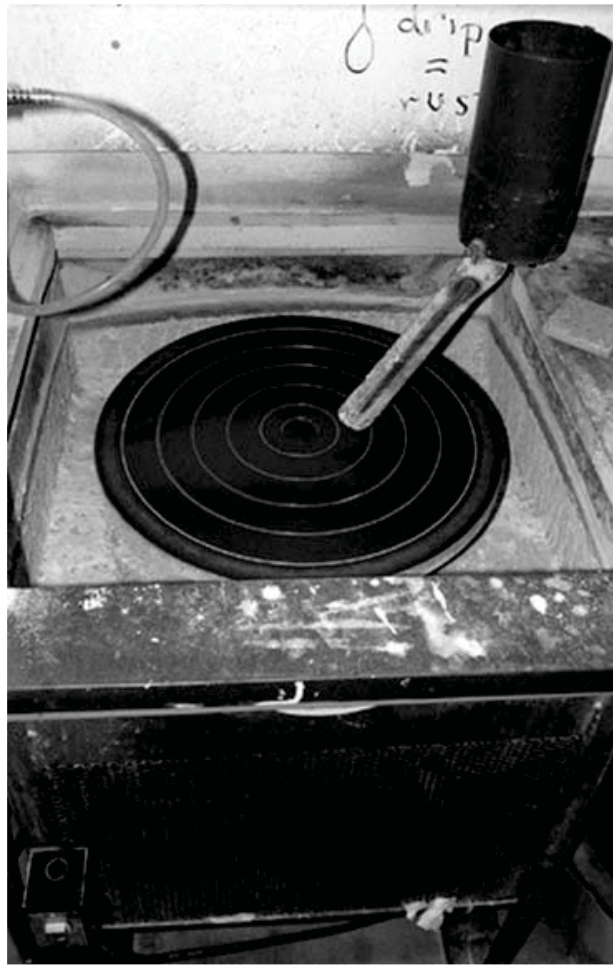
Figure 3-6: Diamond Pacific rotating lap with water drip apparatus
