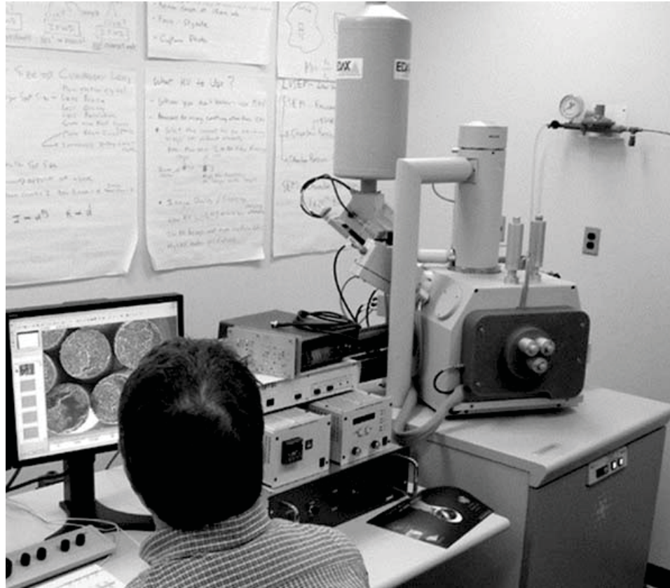
Figure 3-15: FEI/Phillips XL40 Environmental Scanning Electron Microscope
