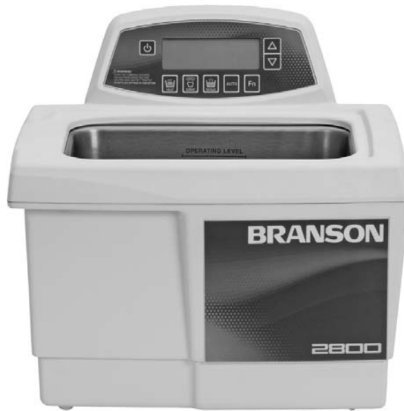
Figure 3-2: Branson Bath Sonicator CPX2800H
