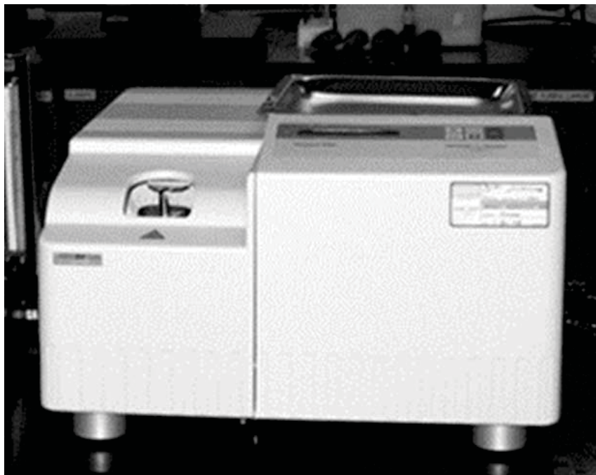
Figure 3-10: Mettler Toledo 823E Differential Scanning Calorimeter
