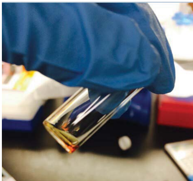
Figure 2-1. Image of the experiment to determine the cure time of adhesive. The cure time was determined when the adhesive solution stopped flow in a tilt vial. 8
