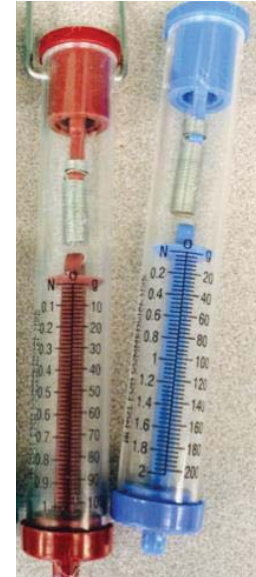
Figure 9: Spring gauges used for the lab lift and drag force (Image by author, 2015)
