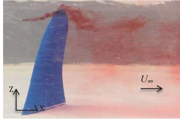
Figure 76: Profile view of the SFPW at \alpha = 45^\circ , U_\infty = 0.5\text{mps} using dye injections at the fin tip
