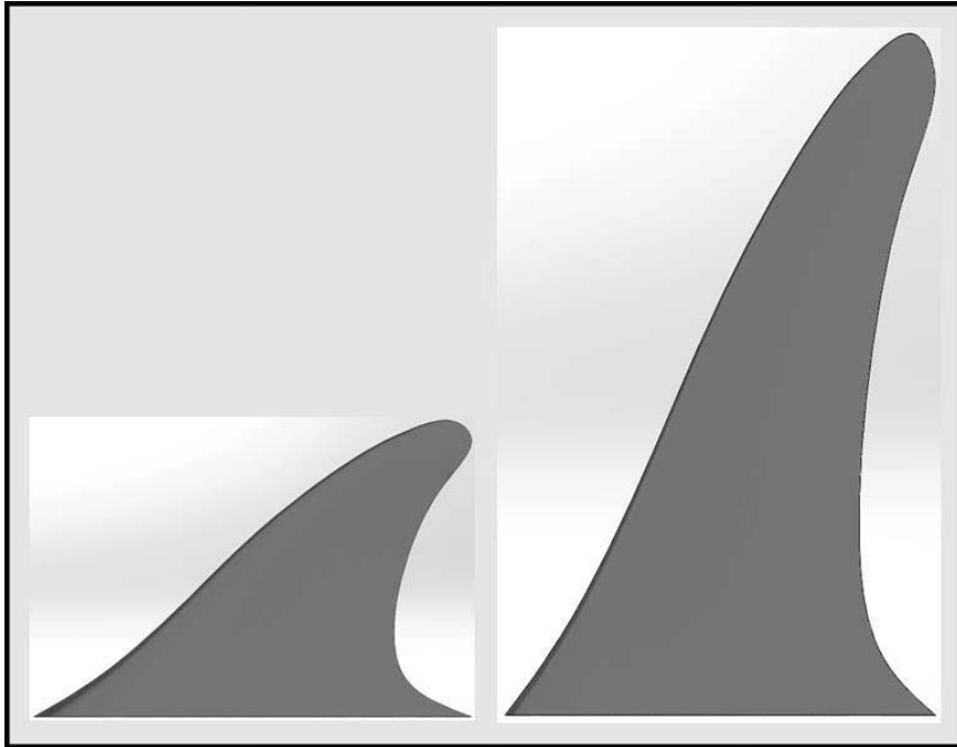
Figure 92: Fin Whale profile view, [left] original design L_w=112.0\text{ mm} L_h=76.15\text{ mm} , [right] full-scaled design L_w=112.0\text{ mm} L_h=177.8\text{ mm}
