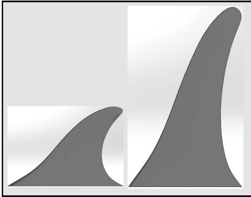
Figure 95: Pacific Spotted Dolphin profile view, [left] original design L_w=112.0 mm L_h=77.44 mm, [right] full-scaled design L_w=112.0 mm L_h=177.8 mm
