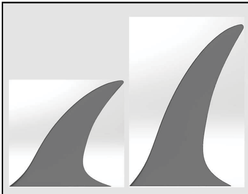
Figure 98: Swordfish profile view, [left] original design L_w=112.0 mm L_h=116.38 mm, [right] full-scaled design L_w=112.0 mm L_h=177.8 mm
