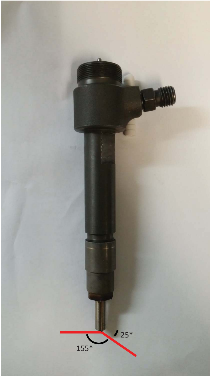
Figure 12-1: Bosch 7 Hole Common Rail Injector Spray Angle
