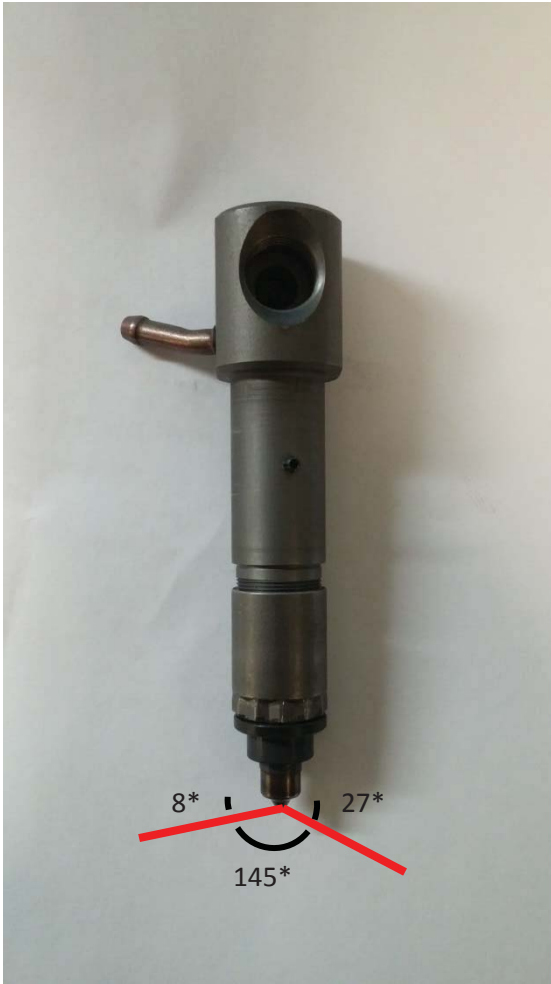
Figure 12-2: Yanmar L100V 5 Hole OEM Injector Spray Angle
