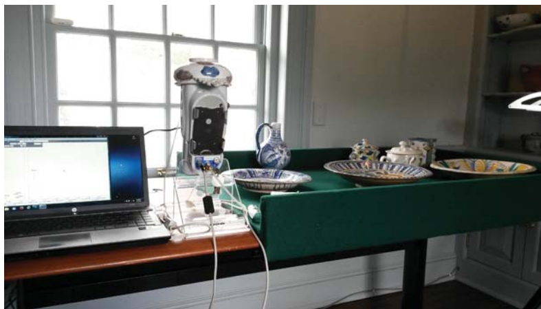
Figure 1.2 Basic instrument setup with complete software package, vacuum pump, and instrument stand.
