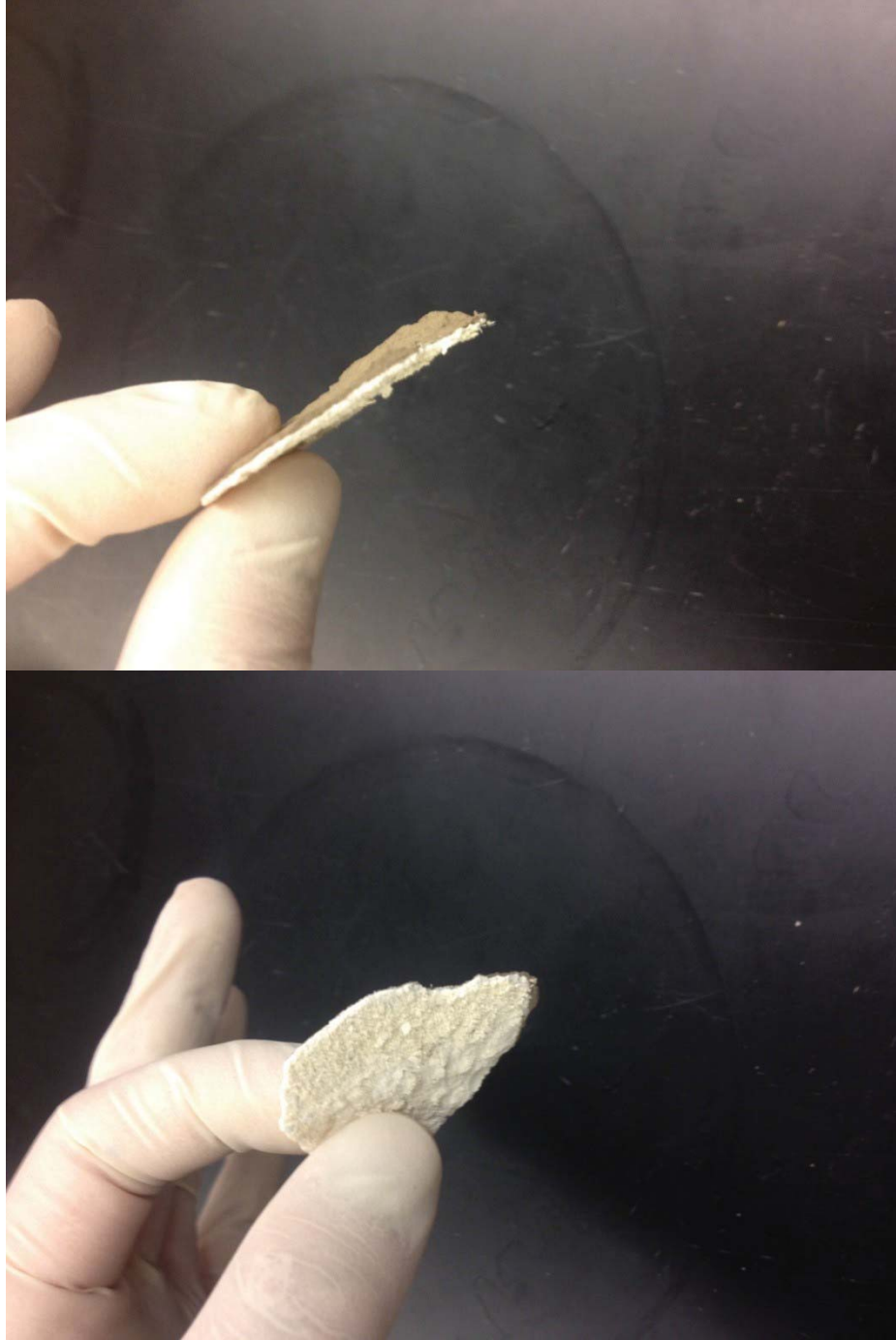
Figure 5.2: Solid white precipitate crust from R1. Note the iron mine tailings directly beneath the crust.
