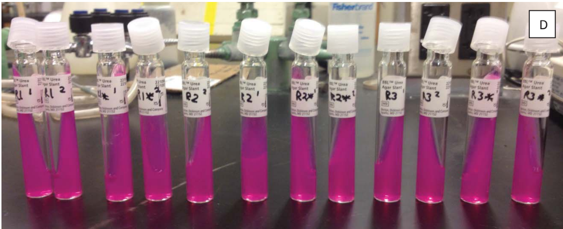
Figure 5.5: Urea - Agar slants after 6 hours of incubation time (A and C) and after 24 hours of incubation time (B and D). All reactors tested positive for urea-degraders. From left to right (in duplicates), R1,R1*, R2,R2*,R3,R3*.
