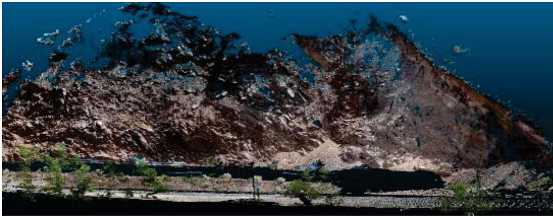
FIGURE 6-10: LiDAR POINT CLOUD GENERATED FOR SLIDE 2. THE ROCK STRUCTURES CAN BE EXTRACTED FROM THIS AND USED FOR ANALYSIS. THE HOLE AT THE TOE OF THE SLOPE IS DUE TO SLOPE ANGLE CHANGES THAT THE LiDAR SCANNER COULD NOT CAPTURE. THIS AREA IS NOT SIGNIFICANT TO THE OVERALL STRUCTURE OF THE SLOPE.
