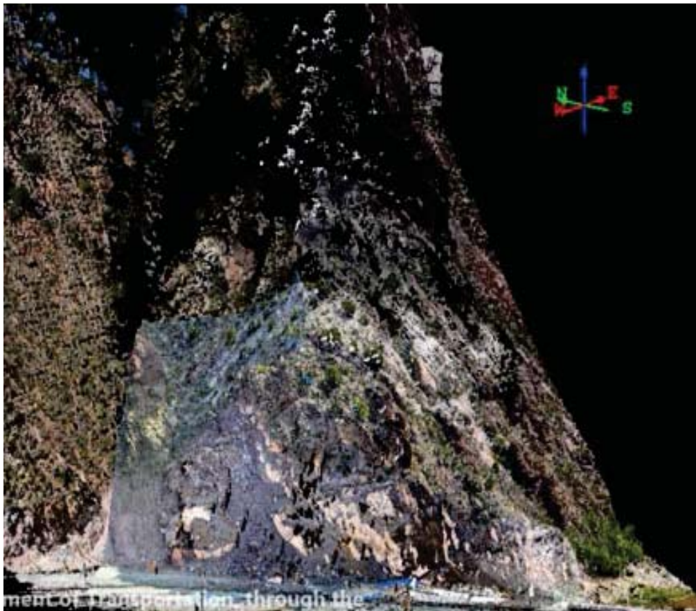
FIGURE 6-6: LIDAR AND OPTICAL PHOTOGRAMMETRY POINT CLOUDS FOR SLIDE 1 ARE COMBINED INTO A SINGLE IMAGE. THE INTEGRATED DATA SETS PROVIDES THE BEST POINT CLOUD FOR USE IN HAZARD ANALYSIS.
