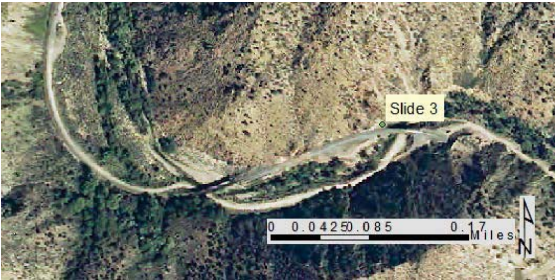
FIGURE 4-4: ZOOMED IN ORTHO-PHOTO OF SLIDE 3. FROM THIS PHOTO, MEASUREMENTS OF "SITE DISTANCE" AND "ROAD WIDTH" CAN BE DETERMINED FOR THE RHRS CATEGORIES.
