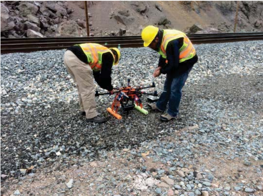
FIGURE 2-7: OPTICAL PHOTOGAMMETRY SET-UP USE AT THE STUDY SITE LOCATION IN SOUTHERN NEVADA. THE CAMERA WAS ATTACHED TO AN UNMANNED AERIAL VEHICLE, TO CAPTURE THE SLOPE FROM ABOVE.
