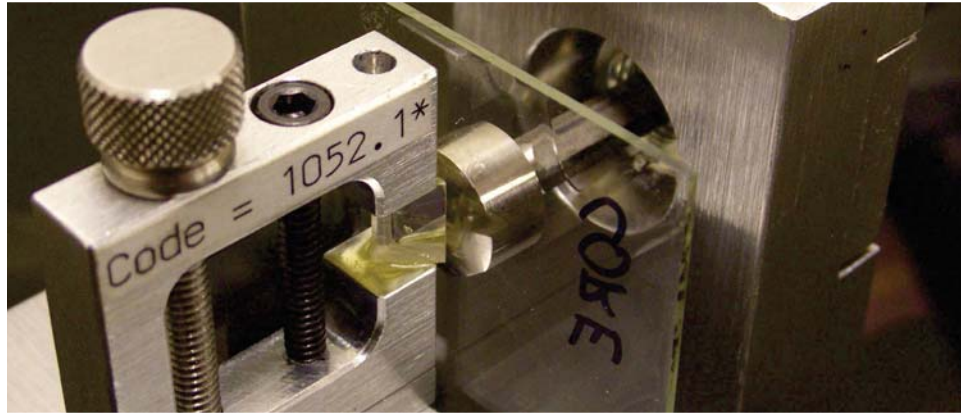
Figure 3.6: Prism coupling method conducted on core material spin-coated on a glass substrate.
