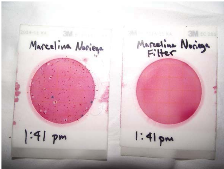
Figure 7. 3M Petrifilms displaying the total coliforms (Red and blue dots) and E. coli (blue dots) in 1 ml of untreated drinking water (left) and filtered drinking water (right) following 24 hours of incubation. This sample was taken from the aqueduct in the town of La Cantero in rural Panama.
