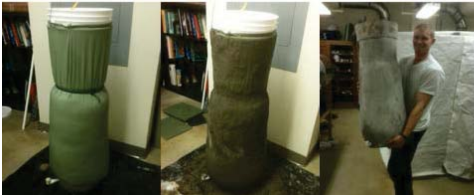
Figure 10. Process of enlarged FBSF construction. The three photos from left to right show the filled cloth mold, the first layer of cement, and the finished shell before the addition of sand, gravel, and the outlet tube. This filter was used alongside a plastic V10 model filter for comparison.
