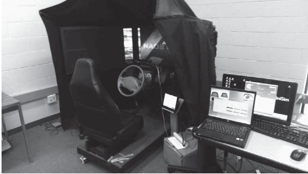
Figure 2. Equipment setup. From left to right, the NADS simulator, the tablet and stand used during physical distraction, Facelab 4.5 laptop.
