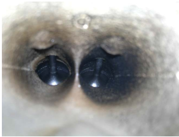
Figure A-3. Intake valves of Ecotec 2.0L turbo GM engine
