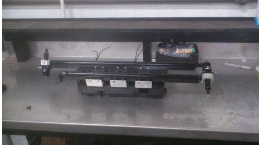
Figure A-9. PFI injector complete mounting.
